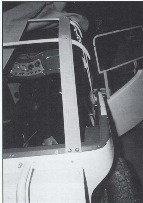
Fasten the top straps to the top rail half way between the front and rear edge. Leave the excess at this time. The copper top bow socket is visible with the crimped tabs.
